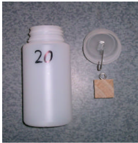
Figure 1: Testing flask and cube of wood used as the test-piece
